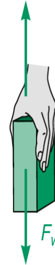
(a) The upward force of the hand equals the downward force of the weight.
