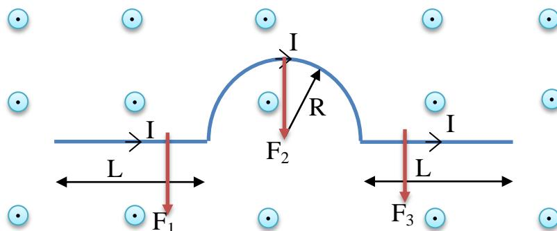
$$F_1 = F_3 = I L B \sin 90^\circ = I L B \quad (\text{down})$$
