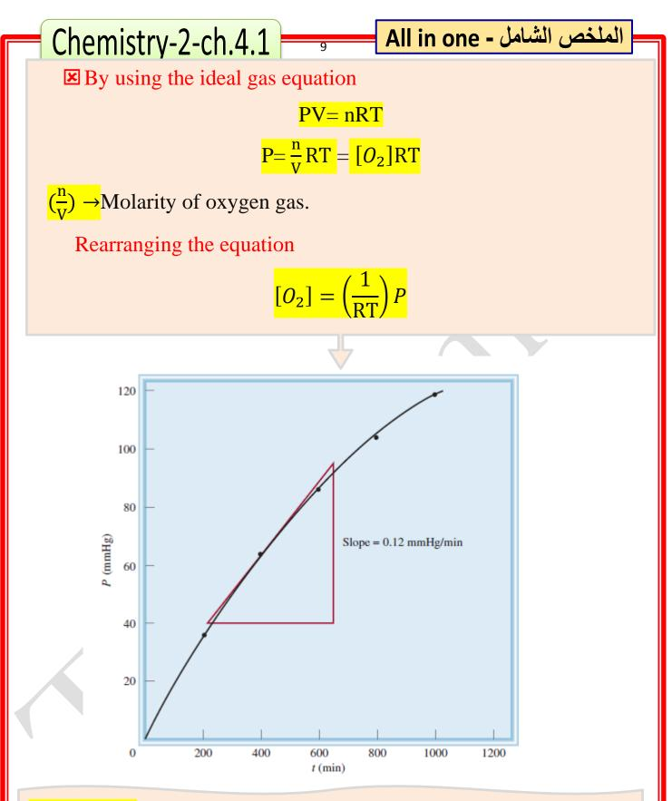
Figure show: The instantaneous rate for the decomposition of hydrogen peroxide at 400 min is given by the slope of the tangent multiplied by 1/RT. The reaction rate " rate of oxygen production"
